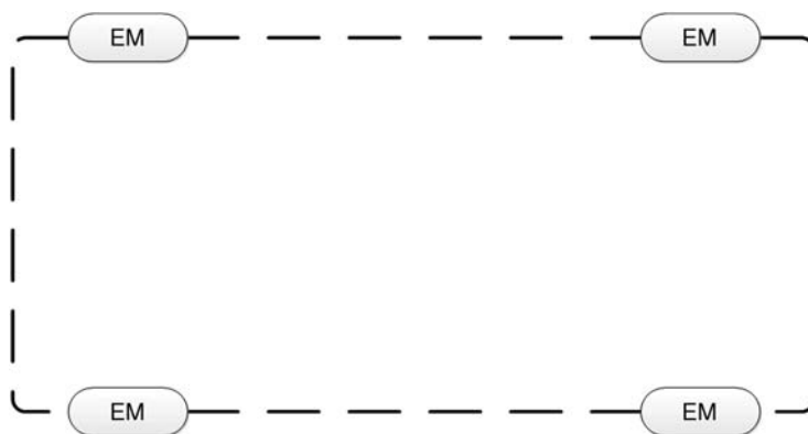
Figure 2.8 In-wheel motor all-wheel drive on an electric powertrain arrangement. Note: EM = electric motor
