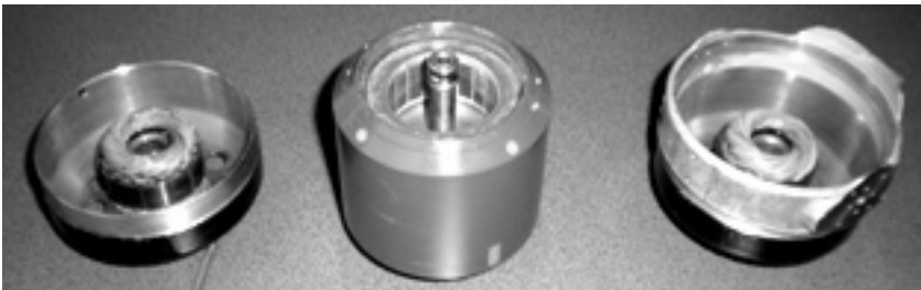
Figure 1.14 3.68 kW (5 HP), 3200 Hz (62,000 rpm) induction motor with forced liquid cooling: a) high speed gyroscope dual IM with outer rotor, b) high speed gyroscope dual IM with outer rotor
