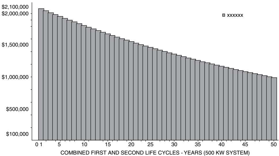
Figure 8.40. SAM solar power system 50-year life cycle energy production graph.
