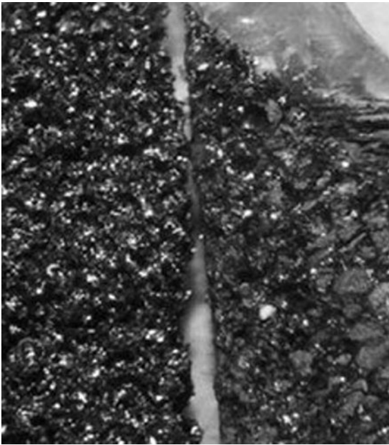
Figure 12.13. Foam-based battery used electrode. Source: Photo courtesy of Firefly Energy
