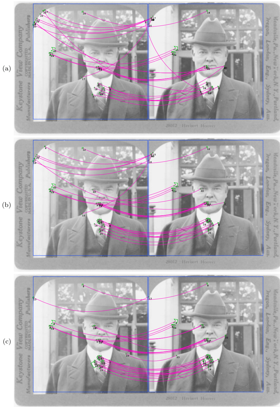
Figure 7.31 Rejection of weak or ambiguous matches by limiting the ratio of primary and secondary match distance \bar{\rho}_{\text{match}} (see Eqns. 7.104–7.105). \bar{\rho}_{\text{match}} = 1.0 (a), 0.8 (b), 0.5 (c).
