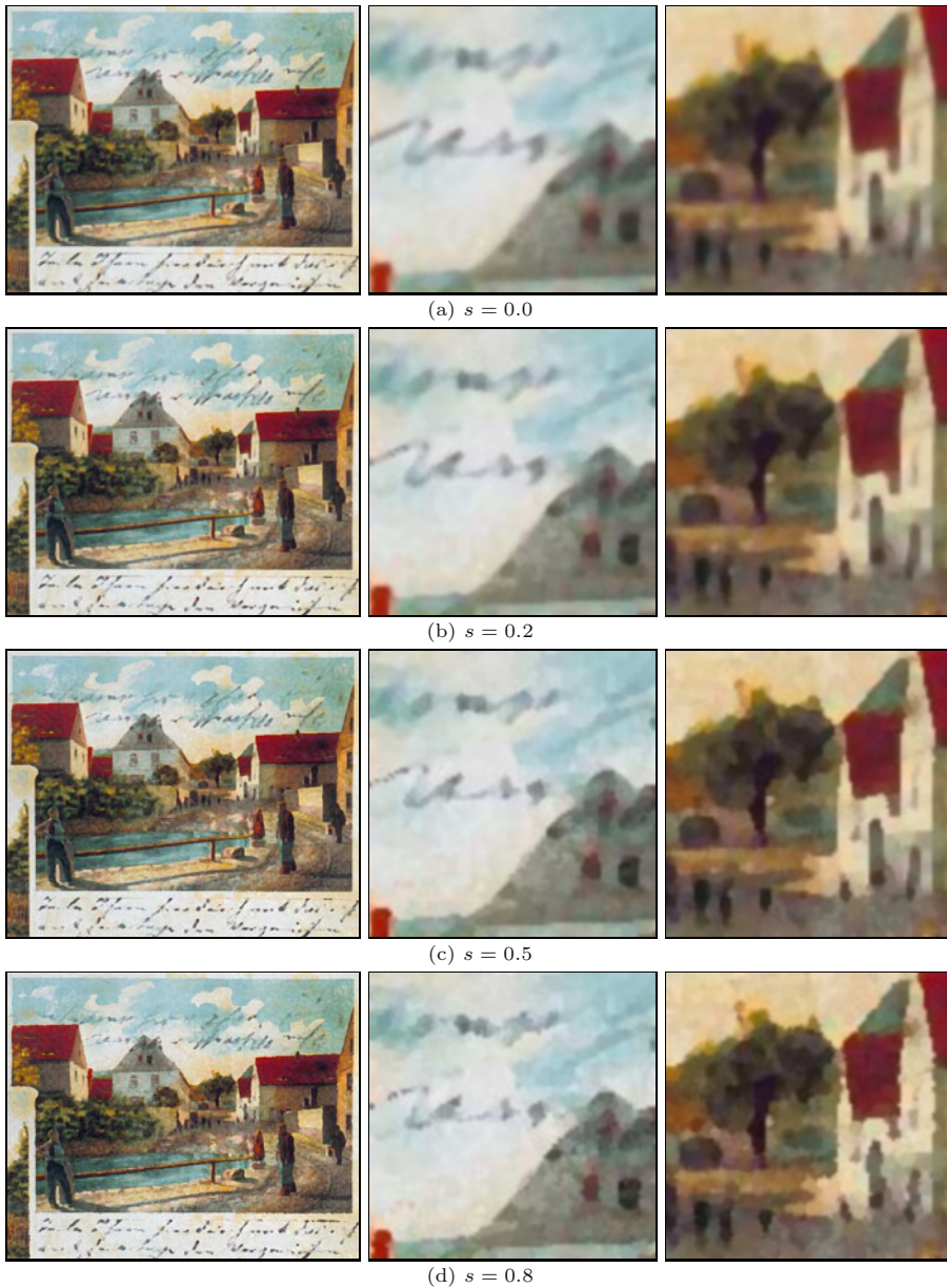
Figure 3.19 Sharpening vector median filter with different sharpness values s . The filter radius is r = 2.0 and the corresponding filter mask contains n = 21 pixels. At each pixel, only the a = 21, 17, 12, 6 closest color samples (for sharpness s = 0.0, 0.2, 0.5, 0.8 , respectively) are considered when calculating the local vector median.
