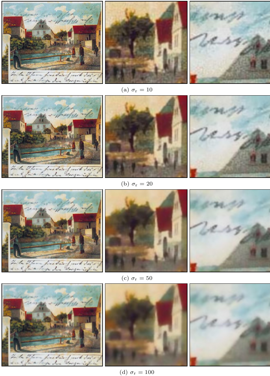
Figure 5.9 Bilateral filter—color example. A Gaussian kernel with \sigma_d = 2.0 (kernel size 15 \times 15 ) is used for the domain part of the filter; working color space is sRGB. The width of the range filter is varied from \sigma_r = 10 to 100. Original image in Fig. 5.3 .
