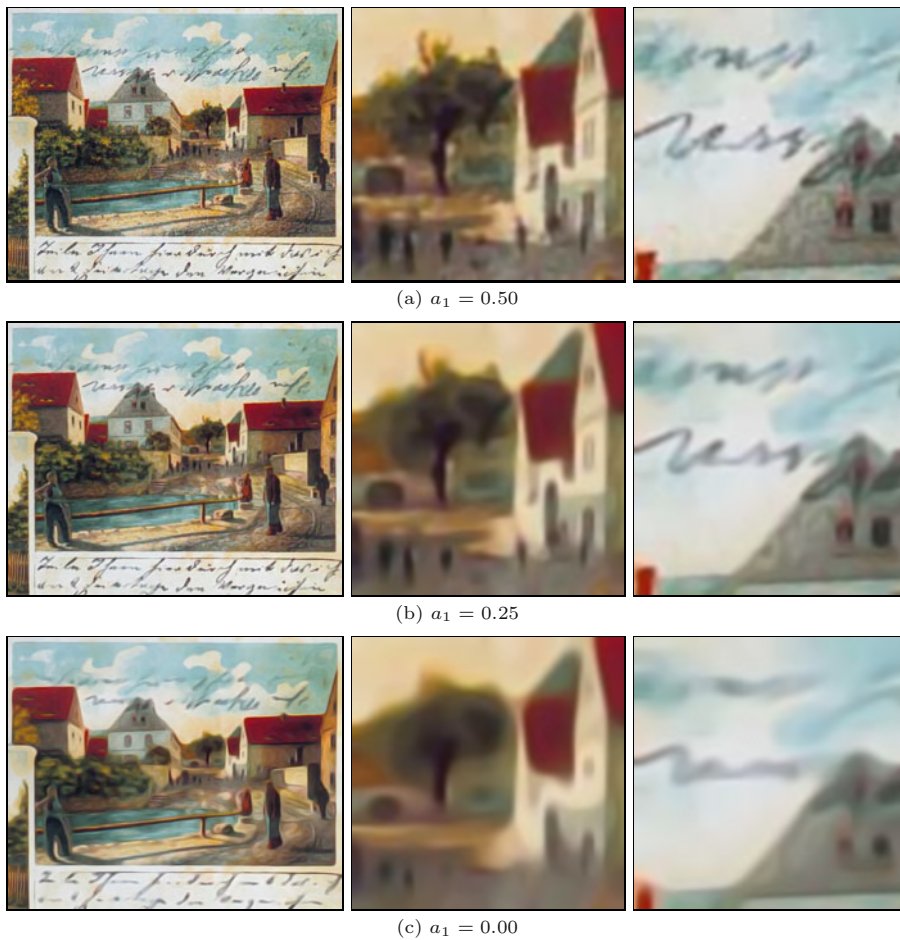
Figure 5.20 Tschumperlé-Deriche filter example. The non-isotropy of the filter can be adjusted by changing parameter a_1 , which controls the diffusion along contours (see Eqn. (5.73)): a_1 = 0.50, 0.25, 0.00 (a-c). Parameter a_2 = 0.90 (constant) controls the diffusion in the direction of the gradient (perpendicular to contours). Remaining settings are T = 20 , d_t = 20 , \sigma_x = 0.5 , \sigma_s = 0.5 (see the description of Alg. 5.9 ); original image in Fig. 5.3 .
