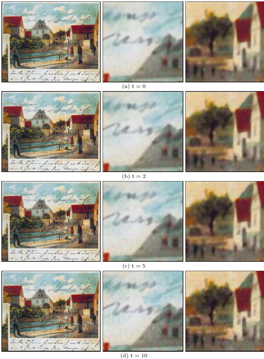
Figure 3.20 Sharpening vector median filter with different threshold values t = 0, 2, 5, 10 . The filter radius and sharpening factor are fixed at r = 2.0 and s = 0.0 , respectively.
