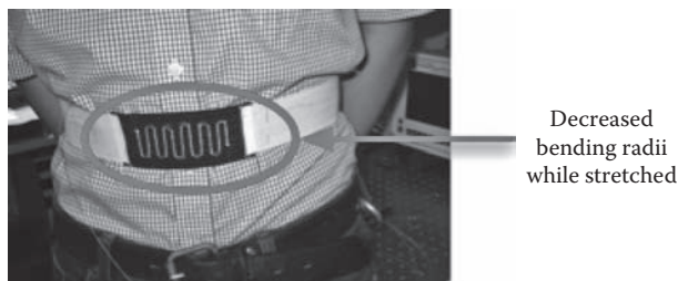
FIGURE 2.10 Monitoring of respiratory abdominal movement of an adult by polymer optical fiber optical time-domain reflectometry.
