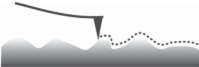
Fig. 2. In contact mode, the tip follows directly the topography of the surface while it is scanned.
