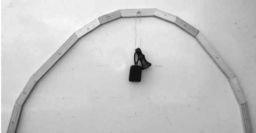
Figure 11.3: Photograph showing an inverted arch in compression.
