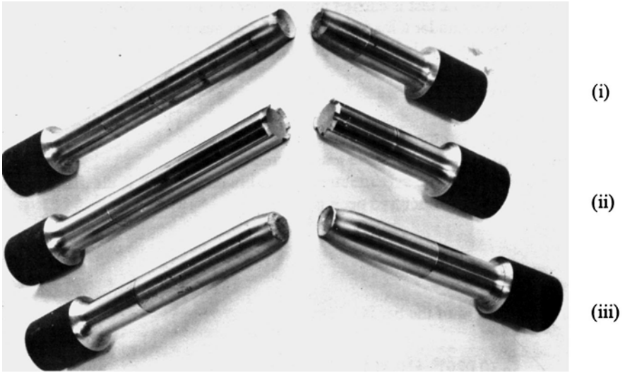
Figure 1.11 Tensile failures in steel specimens showing necking in mild steel, (i) and (iii), and brittle fracture in high-strength steel, (ii).
