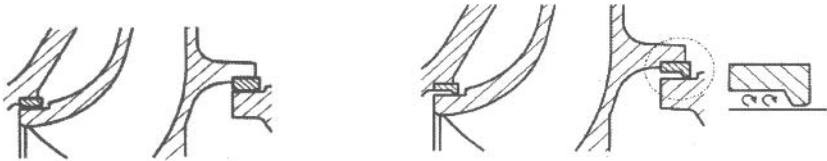
Figure 11.5: Conventional wear ring profiles (left) and enhanced contour wear rings (right). Source: Ref. 3.
