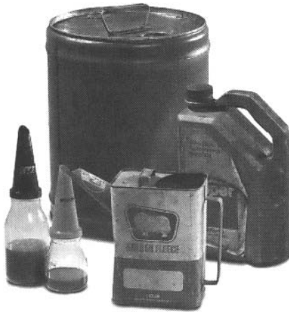
Figure 12.2: Unsuitable lube transfer containers.
