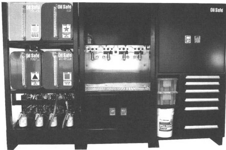
Figure 12.8: Modern lubrication work center (2010).
