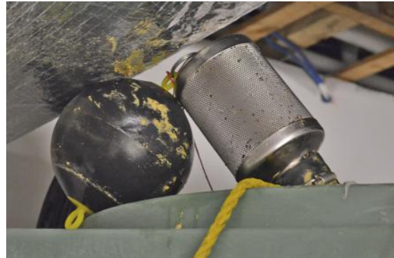
Figures 5.8a and b A floating extractor clogged with pollen after removal from the tank (a), and then later after cleaning and removing the pollen (b).
