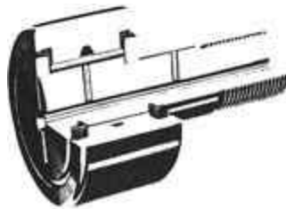
FIGURE 8.2. Commercial roller follower (needle bearing) (Courtesy of McGill Manufacturing Co., South Bend, Indiana).
