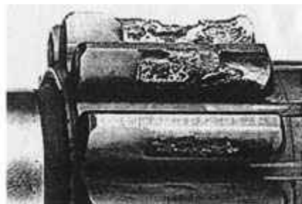
(b) Severe pitting and spalling
