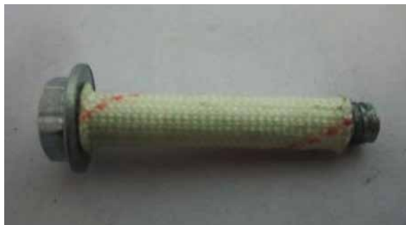
Figure 28. Isolation of screw in a laminated core
