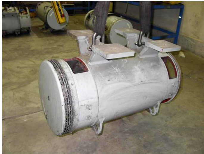
Figure 84. A rotary inverter consists of a mechanically coupled motor and generator
