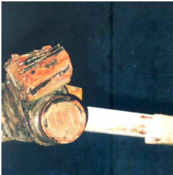
Figure 83. A stator bar with blocked cooling channel
