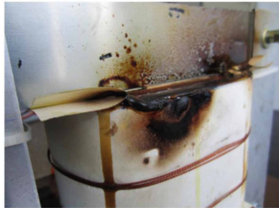
Figure 17. Transformer damage in high temperature test
