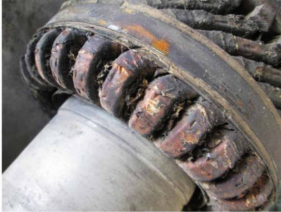
Figure 89. Effect of humidity of winding isolation
