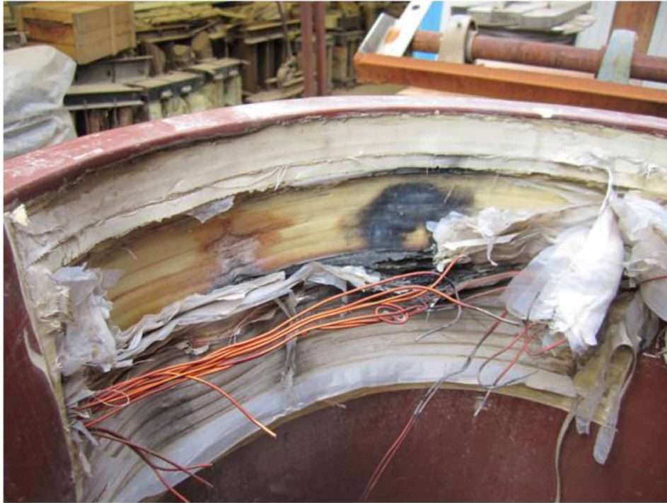
Figure 48. Damaged winding of an air gapped inductor due to electrical breakdown
