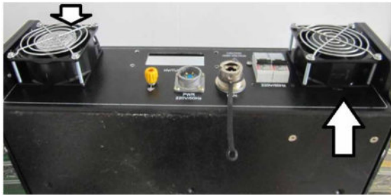
Figure 7. Correct direction of fans in an equipment
