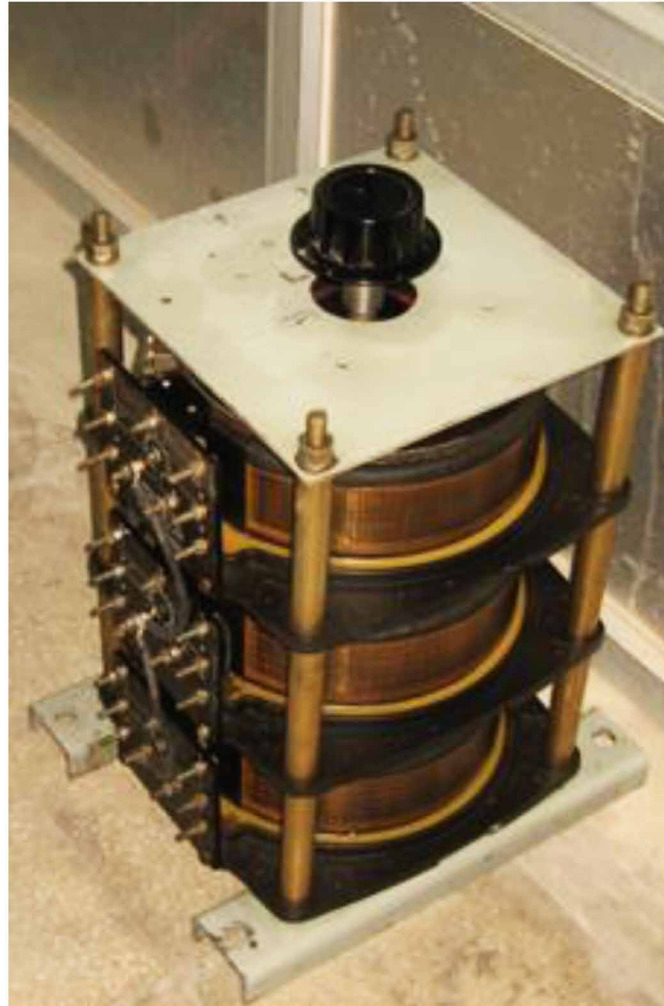
Figure 97. A three phase autotransformer
