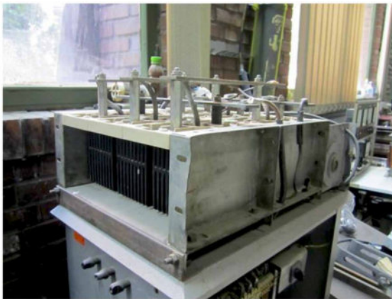
Figure 18. A rectifier with non-isolated heat-sinks
