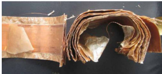
Figure 87. A damaged winding due to humidity
