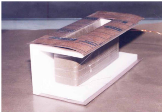
Figure 39. High voltage winding of the transformer with high voltage output
