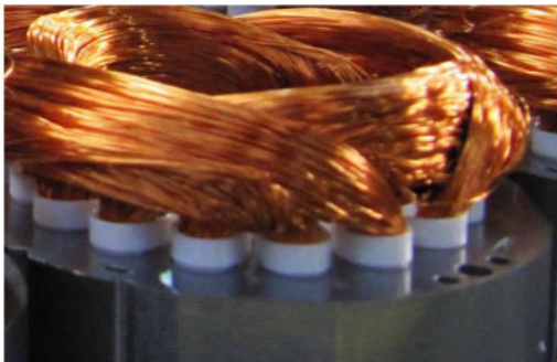
Figure 54. Solid isolators used for isolation between winding of a motor and its core
