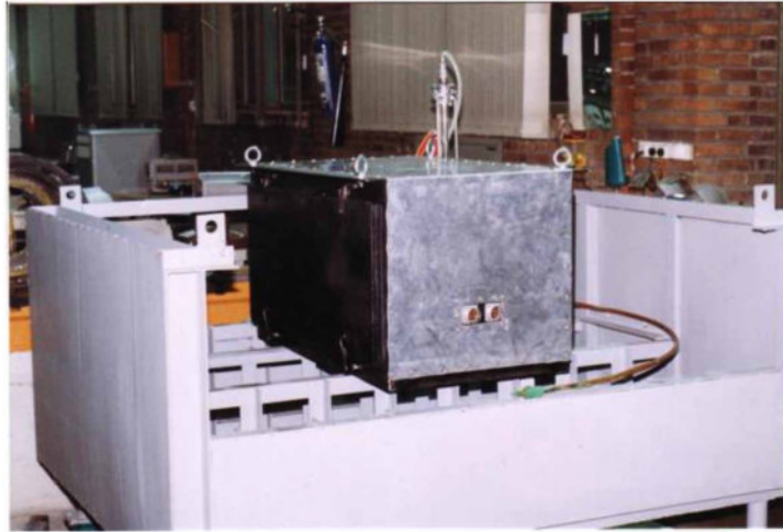
Figure 47. IP test of a converter
