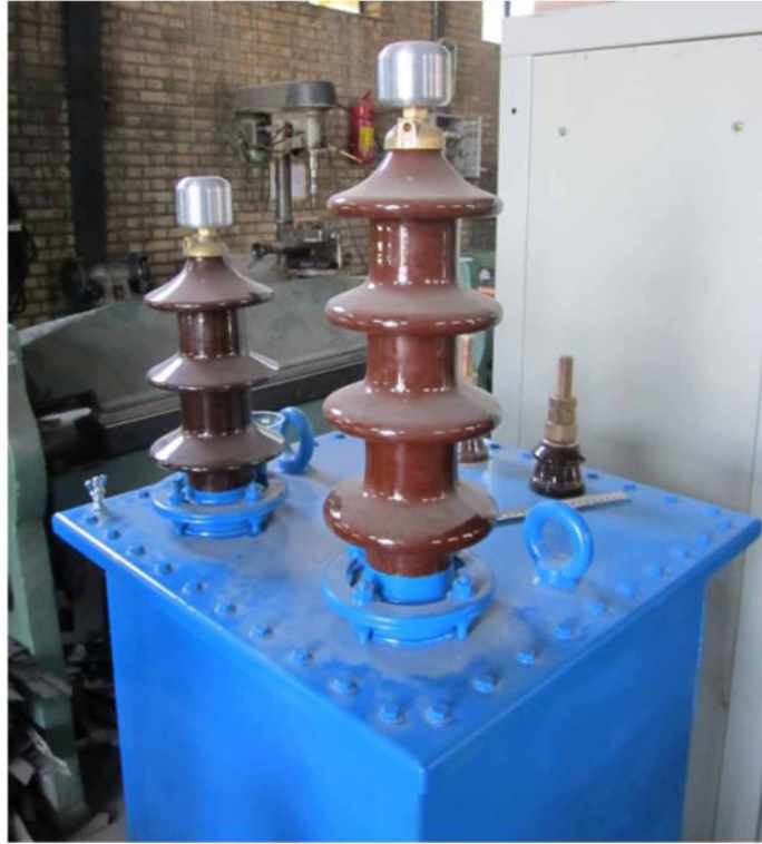
Figure 50. Round head of a high voltage transformer
