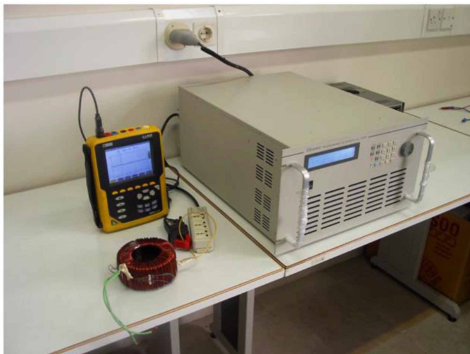
Figure 37. A harmonic generator using for EMI tests
