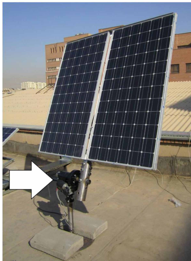
Figure 53. A servo motor used in sun tracking system of a solar panel
