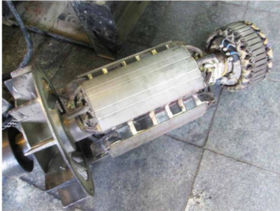
Figure 62. Rotor of a synchronous generator
