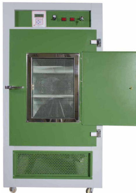
Figure 8. An environmental chamber, (Source: Garouk Co. with permission)
