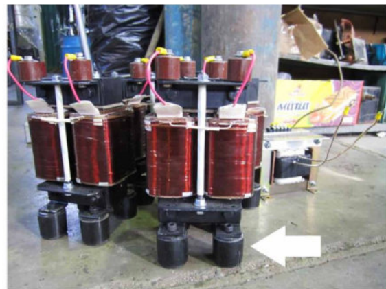
Figure 3. Isolator base for high voltage inductors
