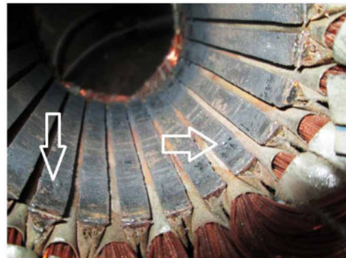
Figure 102. Effect of eccentricity on stator of an induction stator
