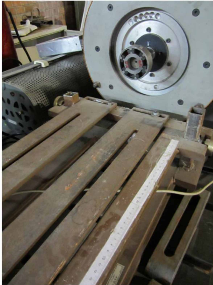
Figure 43. A practical dynamometer
