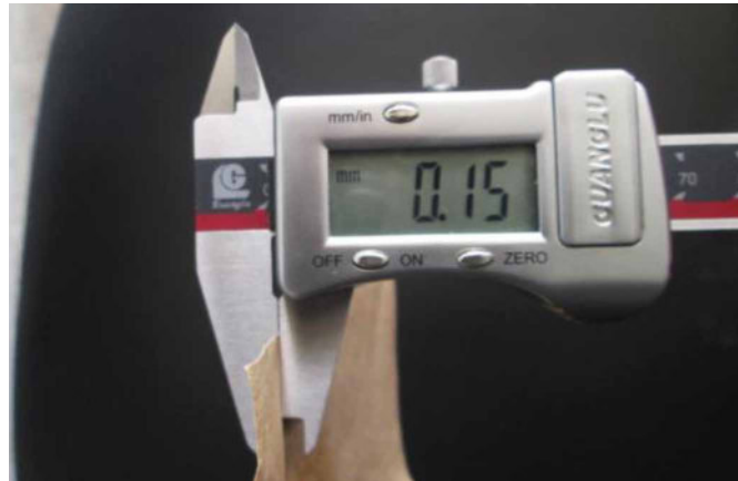
Figure 50. Typical thickness of a thick solid isolator
