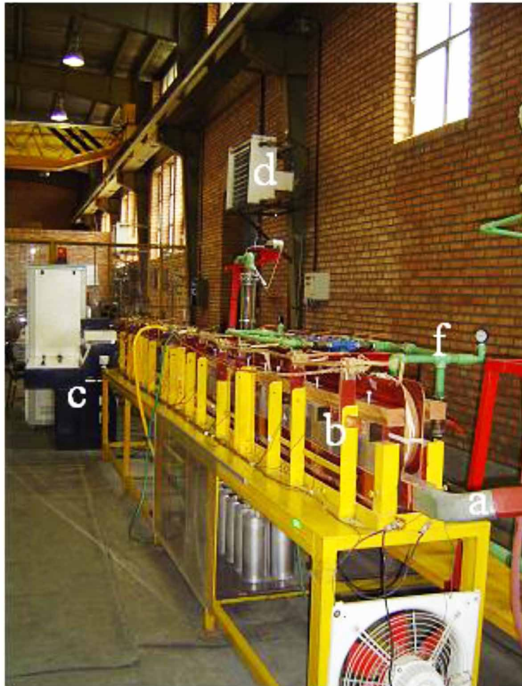
Figure 6. Laboratory experimental setup, (a): stator bar, (b): stator core, (c): temperature measuring equipment, (d): cooler, (f): water cycle
