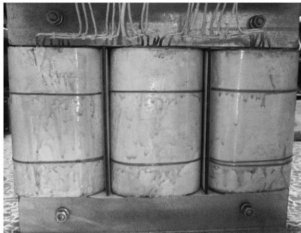
Figure 94. A three phase transformer, Source: Seraj Co. (with permission)
