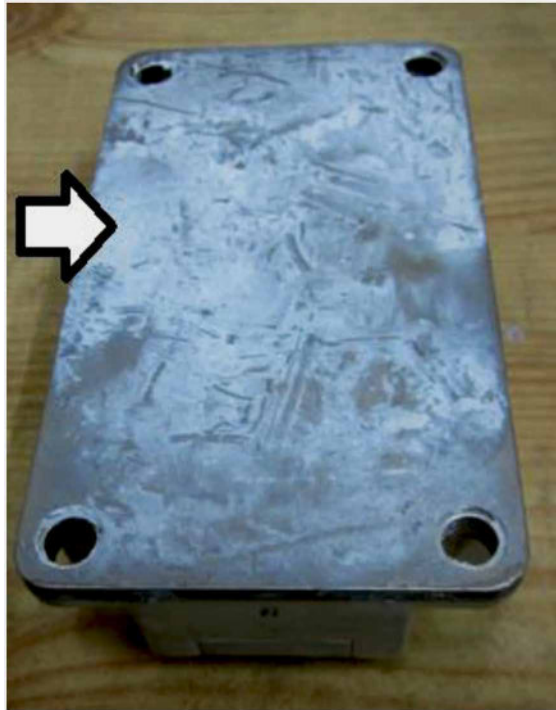
Figure 17. Application of thermal grease on an IGBT
