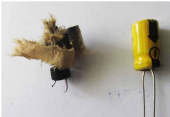
Figure 71. A damaged electrolyte type capacitor with overvoltage
