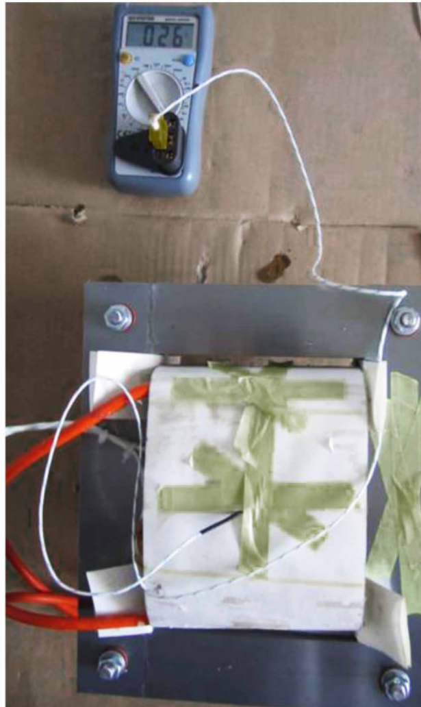
Figure 11. Temperature measurement of a transformer
