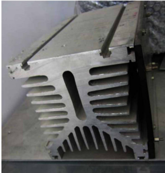
Figure 13. A high performance heatsink
