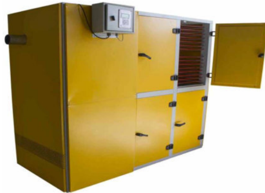
Figure 8. An environmental chamber, (Source: Garouk Co. with permission)
