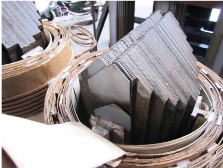
Figure 32. A real transformer with laminated core
