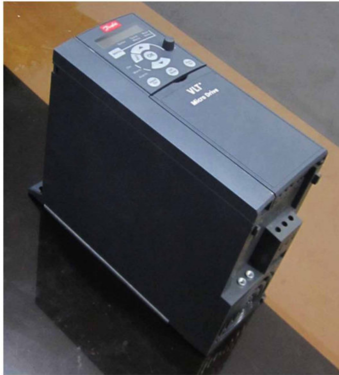
Figure 37. A harmonic generator using for EMI tests
