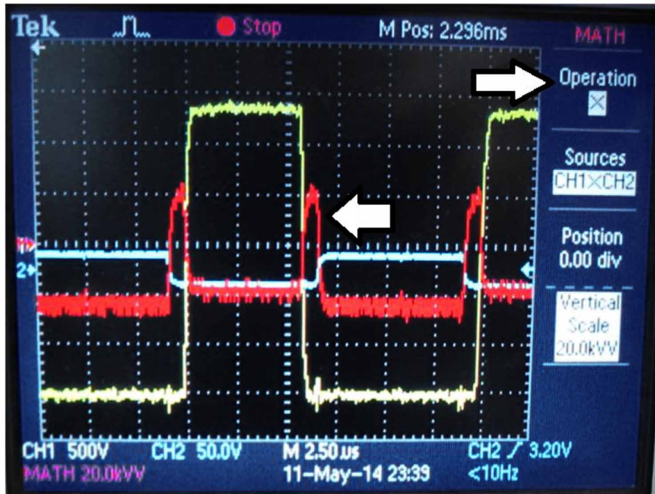
Figure 8. Calculation of switching losses with TEK oscilloscope
