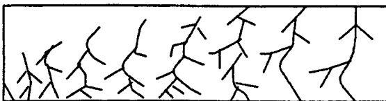
Fig. 8.4 Development of the main or return stroke
