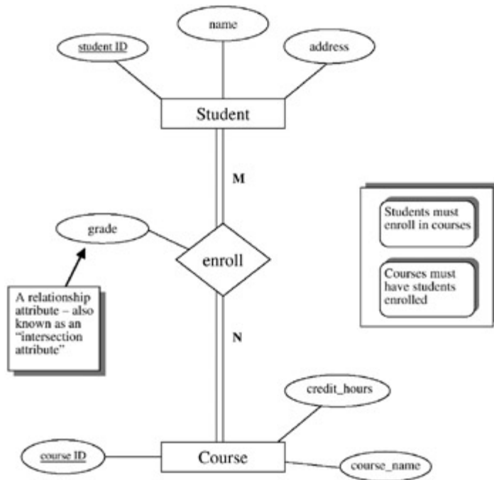
Figure 6.1: An ER Diagram of an M:N Relation with an Attribute of a Relationship
