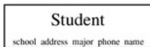
Figure 2.2: An ER Diagram with One Entity and Five Attributes, Alternate Models (Batini, Ceri, Navathe)
