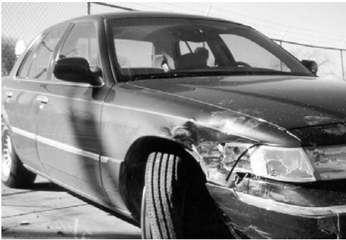
Fig. 1.68 The Car and Right Front Damage
