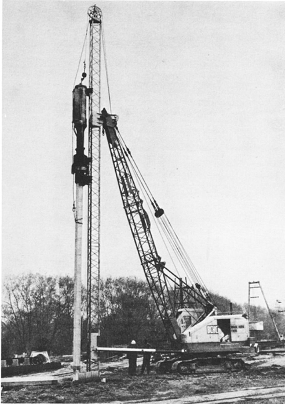
Fig. 3.6 BSP International Foundations Ltd. TL type triangular hanging pile leaders (shown with BSP V.15 double-acting diesel hammer)
