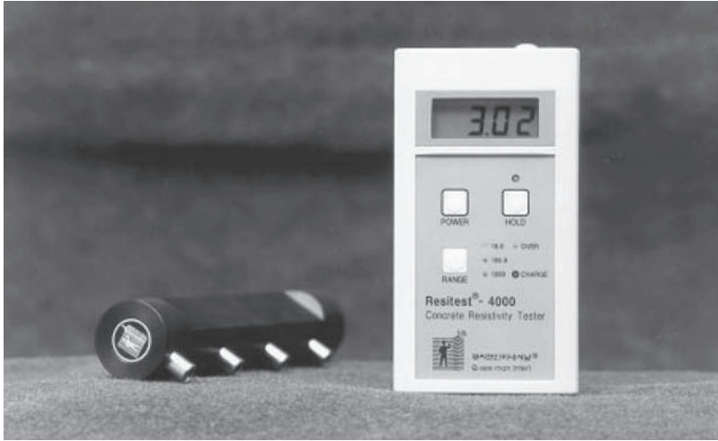
FIGURE 4.28 Electrical resistivity measurement equipment.
