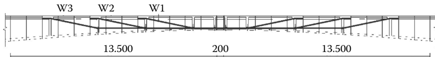
Figure 5.50 Layout of the preparatory external tendons in the continuous rigid frame of Sutong Bridge approach spans.
