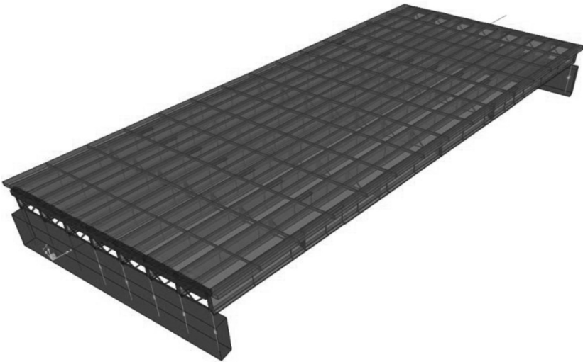
Figure 7.37 Global model of I-270 Middlebrook Bridge.
