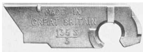
FIGURE 11.2 Typical link of traveling grate.
