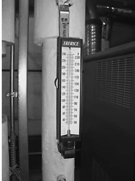
FIGURE 3-31 Photograph of a liquid-in-glass thermometer.
