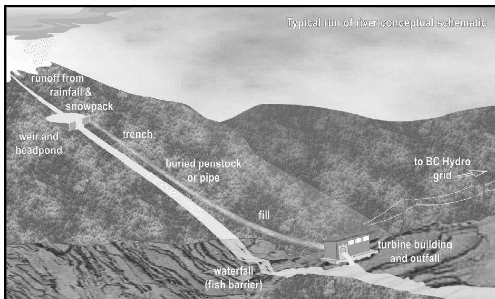
Exhibit 7.79: Schematic of a Typical Run-of-River Facility
