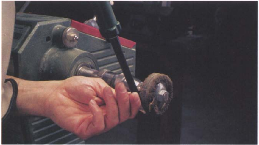
Mount the wheel and arbor in a drill chuck in the lathe.
