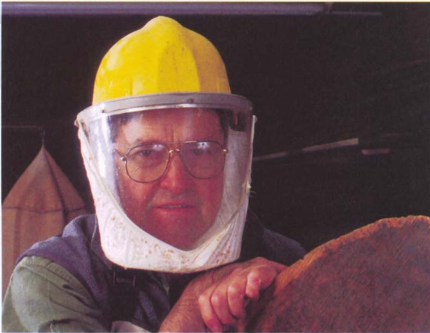
An air helmet offers the best all-around eye and dust protection to the turner. Ear protectors may also be added to this helmet for noisy situations.
