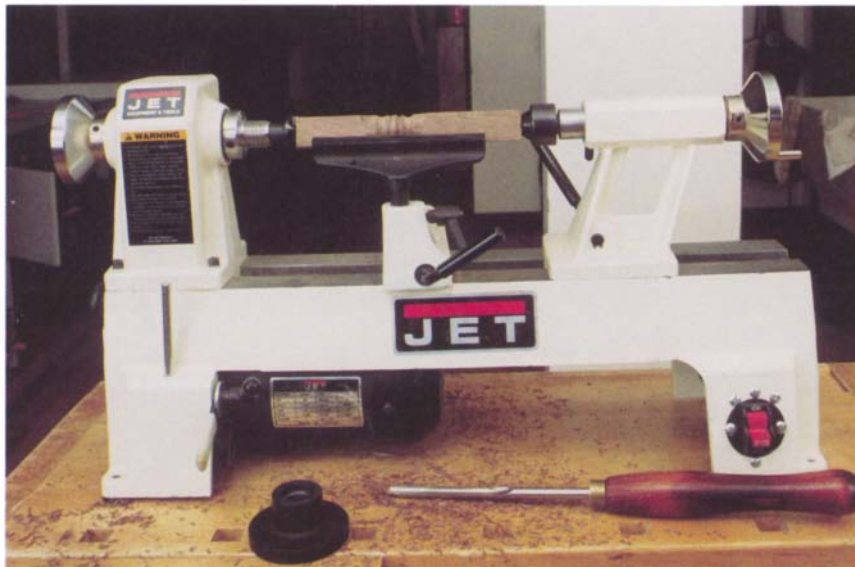
The Jet is typical of today's so-called mini lathes. In reality, it is a short bench lathe with a 10-in. swing and 14 in. between centers. At 78 lb., it is not so portable.
