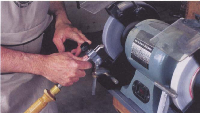
The Sorby fingernail profiling jig is the most economical fingernail grinding jig. The articulated gooseneck part of this jig is actually built by Tormek for Sorby.
