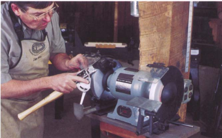
The basic Wolverine jig from Oneway gives you a base unit to mount under each wheel, a tilting table that is good for scrapers, plane irons, and standard woodworking chisels, and an arm (pocket jig) for sharpening roughing gouges and for use with the Vari-Grind jig.
