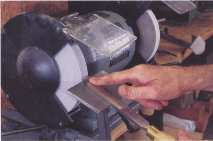
A scraper is one of the easiest tools to grind.
