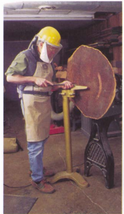
A floor-stand rest allows outboard turning, but you must have a lathe with low enough speed to handle this kind of diameter.
