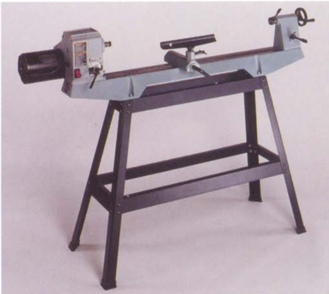
The Delta 46-700 was a groundbreaking lathe when it was introduced in the early 1990s and is still a winner. It offers cast-iron construction where it counts, reasonable swing and between-center distances, and a swing head for larger faceplate work. Best of all, it has variable speed with a low-end speed of 350 rpm. (Photo courtesy Delta.)
