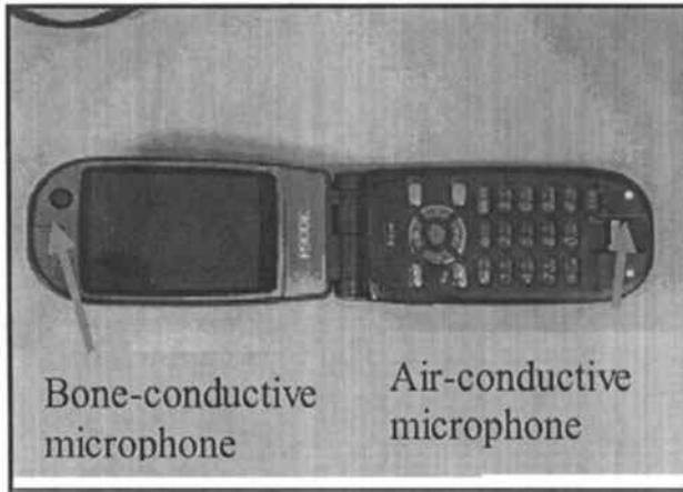
Figure 14-1. Microphone arrangement in mobile device.
