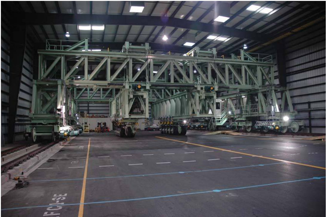
Figure 13.22 Airfield reliability testing at the Hughes Technical Center Pavement Test Facility in New Jersey.
