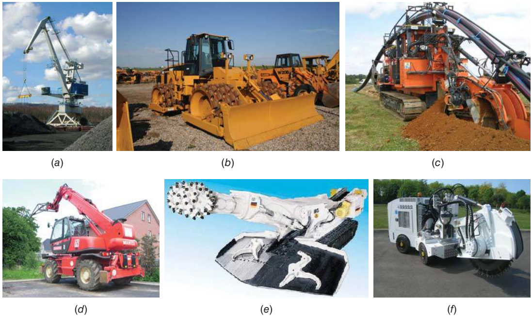
Figure 22.11 Examples of the equipment types typically used for specific work activities: (a) crane, (b) sheepfoot compactor with dozing functionality, (c) excavator with pipe-laying functionality, (d) telescopic handler with crane functionality, (e) road-header machine for tunnel boring, and (f) microtrencher [(a) Lokilech/Wikimedia Commons, (b) Headwater. Equipment/Wikimedia Commons, (c) SA Marais/Wikimedia Commons, (d) Norbert Schnitzler/Wikimedia Commons, (e) FHWA, and (f) SA Marais/Wikimedia Commons].
