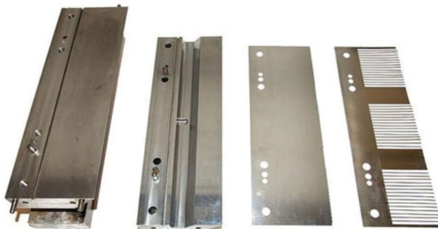
Figure 5.9 Open slot-die head: (from left to right) ink distribution chamber, feed slot, lip and internal mask (shim).
