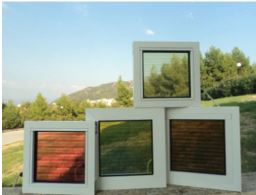
Figure 11.7 Solar windows based on DSSC technology using dyes for fashioning different aesthetic results.
