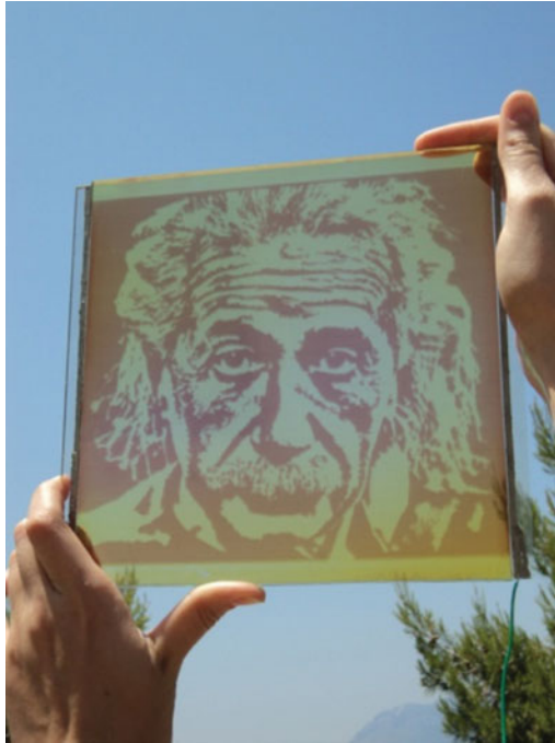
Figure 11.3 Freedom of patterning in DSSC technology by inkjet printing selective components.
