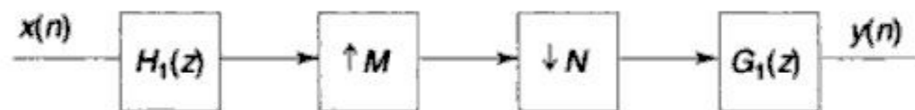
Fig.1.17 Sampling rate conversion for CD to DAT data
