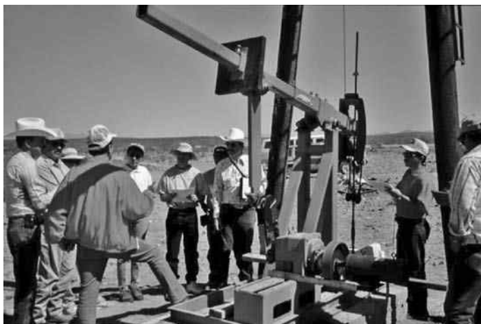
FIGURE 8.41 PV-powered surface jack pump in Chihuahua, Mexico, for a 170-meter deep well.
