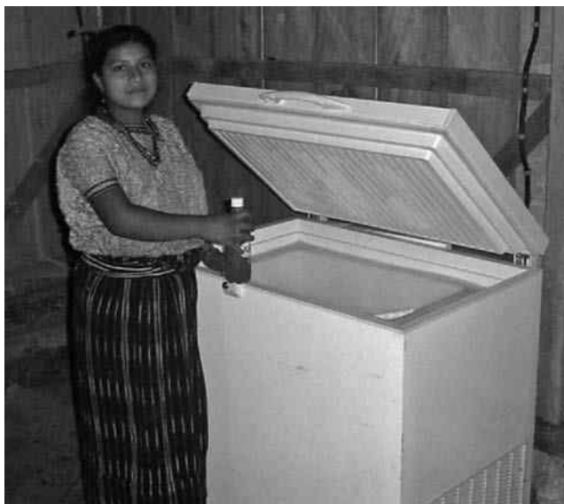
FIGURE 8.26 SunDanzer PV-direct drive refrigerator piloted in the indigenous Mayan village in Quiché, Guatemala, by NASA and Fundación Solar.
