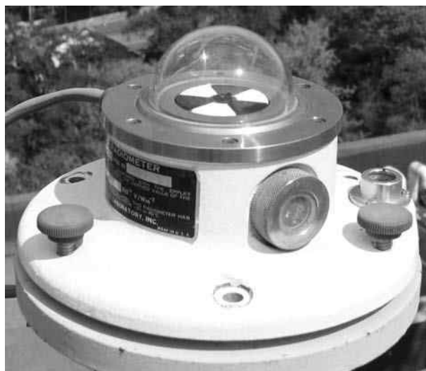
FIGURE 2.25 Pyranometer Eppley Model PSP, first-class reference instrument, as defined by the World Meteorological Organization. (Courtesy of CIE-UNAM.)
