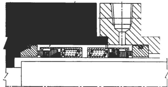
Figure 18. Double seal—back-to-back. (Courtesy of John Crane, Inc.)
