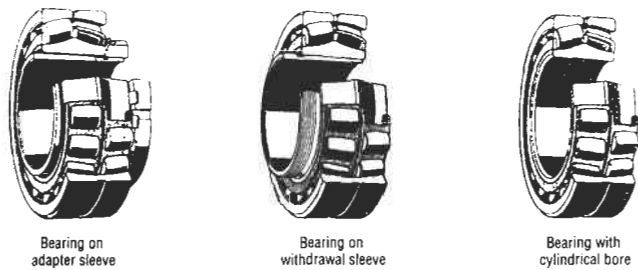
Figure 8. Spherical roller bearings. (Courtesy SKF USA, Inc.)
