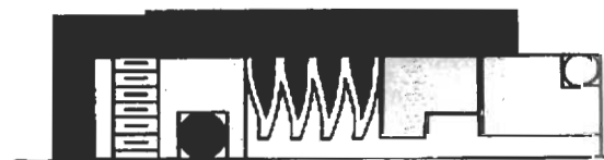
Figure 8. Welded metal-bellows, non-pusher seal. (Courtesy of Durametallic Corp.)
