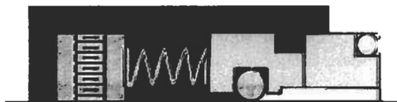
Figure 4. Basic pusher seal. (Courtesy of Durametallic Corp.)
