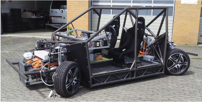
Figure 10.2.: Research vehicle MOBILE constructed as a part of this thesis
