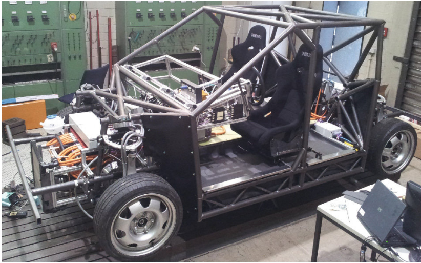
Figure A.6.: MOBILE jacked up at the test bench
