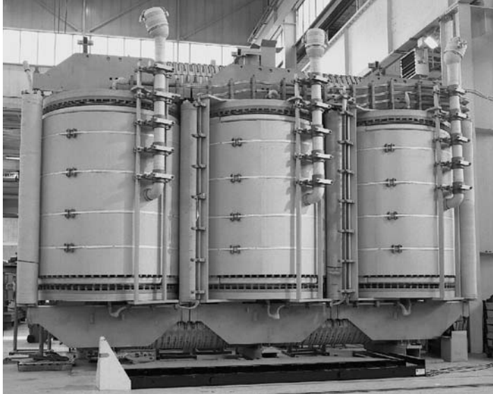
Figure 3.20 A three-phase transformer under construction. Reproduced by permission of TenneT TSO B.V.
