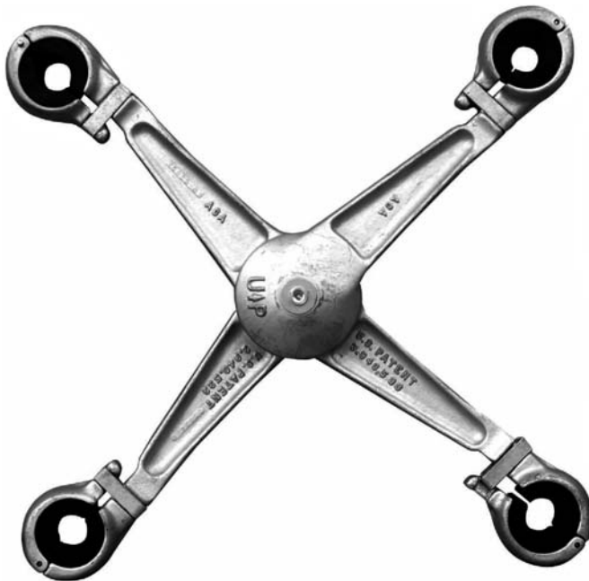
Figure 3.39 A spacer for a four-conductor bundle. Reproduced by permission of Alcoa Conductor Accessories.
