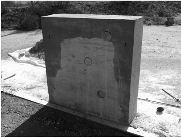
FIGURE 9.1 Shotcrete test panel. (Photo by author, courtesy of Hathaway Dinwiddie Construction Company and Tishman Speyer.)
