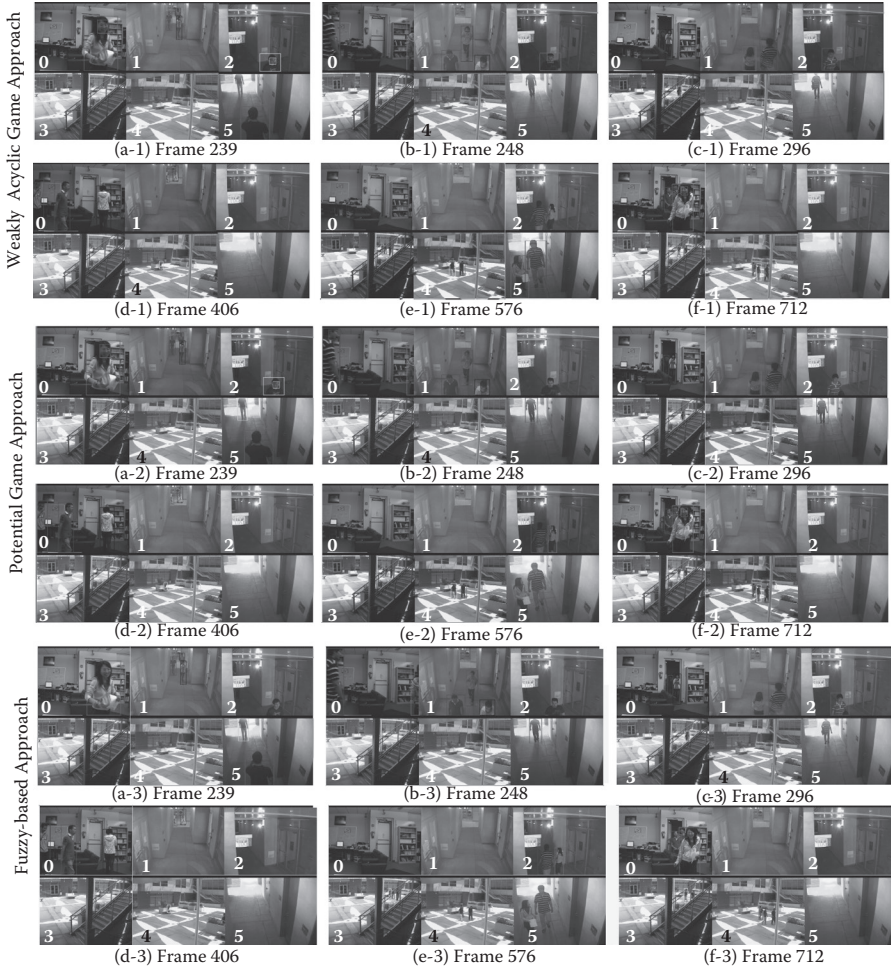
FIGURE 10.7 Experiment #3. Comparison of example frames with different approaches in Case 6. The number is the camera identification. Cameras 1 and 5 served as border cameras. Cameras 0, 1, 2, and 5 handled frontal views. Cameras 3 and 4 were for smooth tracking.
