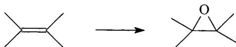
Figure 7.21 Conversion of an alkene to an epoxide with a peroxy acid (RCO 3 H).
