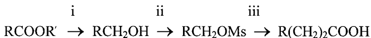
Figure 8.7 Chain extension by two carbon atoms by the malonation route. (i) \text{LiAlH}_4 , (ii) \text{CH}_3\text{SO}_2\text{Cl} (MsCl) etc., (iii) \text{CH}_2(\text{COOEt})_2 etc.
