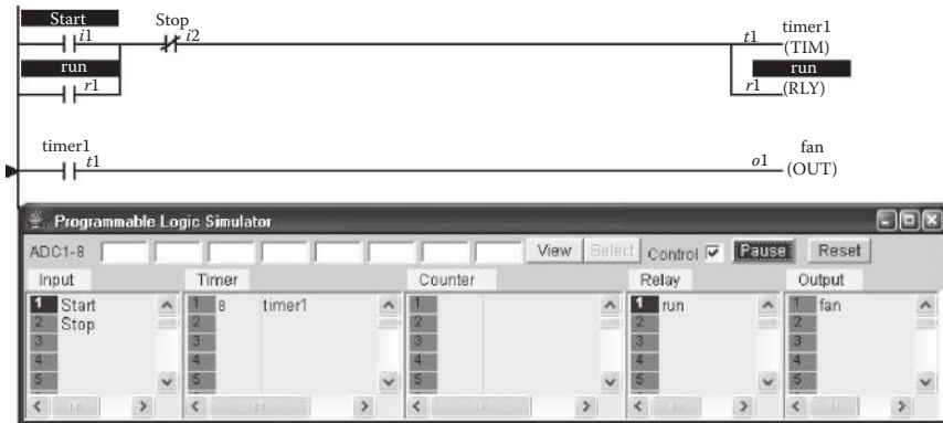
FIGURE 8.11 Start button pressed, delay timer running.
