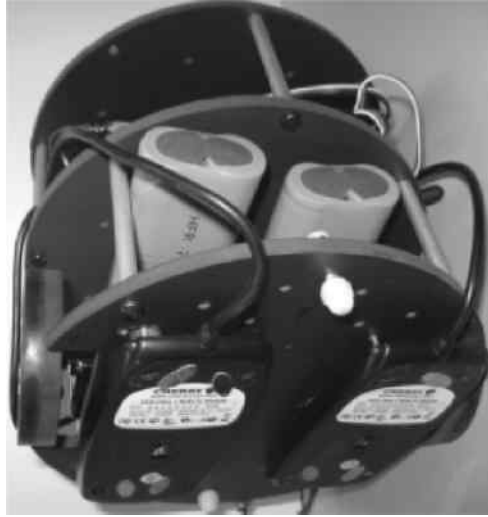
FIGURE 9.21 Optical mice used for odometry.
