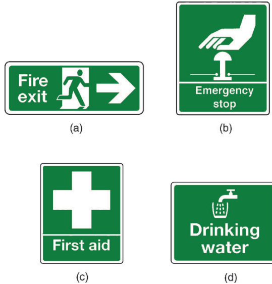
Figure 1.3 Advisory or safe condition signs.
