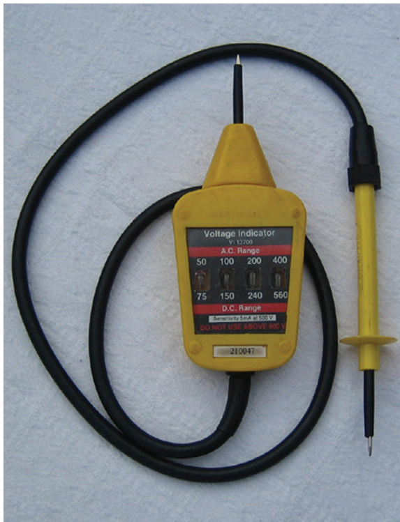
Figure 1.9 Typical voltage indicator.
