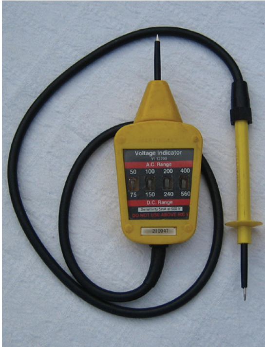
Figure 3.8 Typical voltage indicator.
