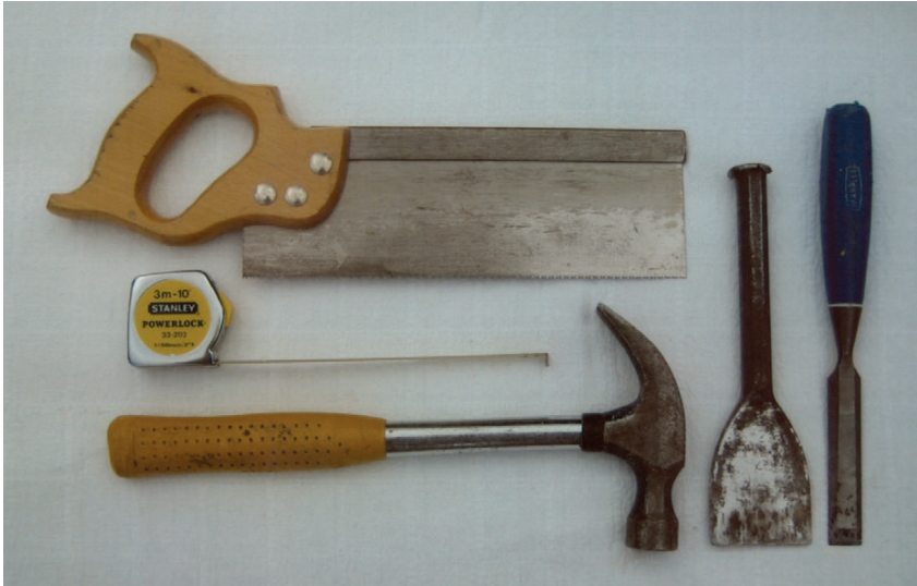
Figure 2.18 Some additional tools required by an electrician engaged in house wiring.
