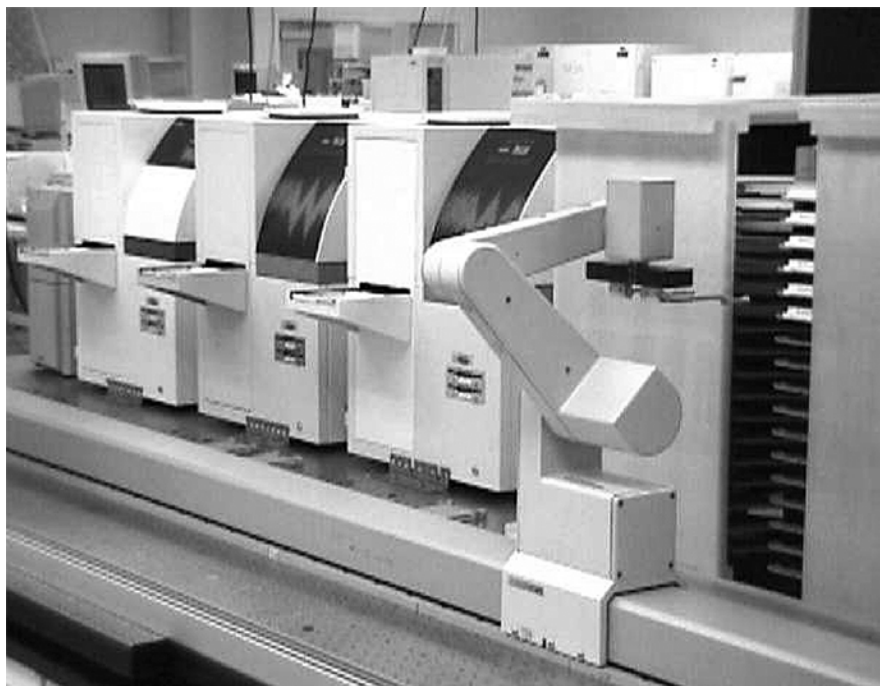
Fig. 4. Scintillation counting workstation.
