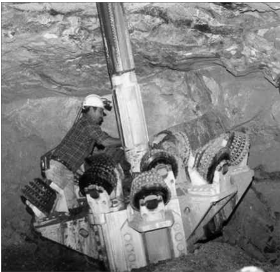
FIGURE 12.2 A reaming head. (Courtesy of Atlas Copco.)
