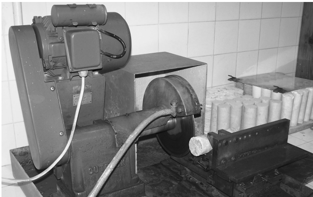
FIGURE 3.2 Typical core diamond sawing machine.
