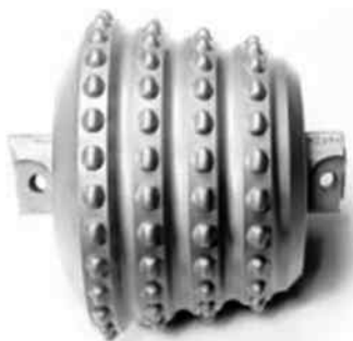
FIGURE 12.5 Cutter preferred to use in hard and abrasive rocks.
