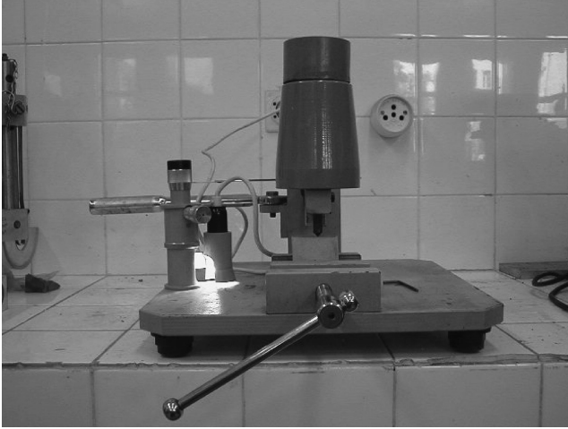
FIGURE 3.11 Typical Cerchar abrasivity device.
