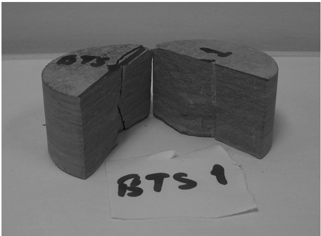
FIGURE 3.8 An example of the normal failure type of BTS testing.
