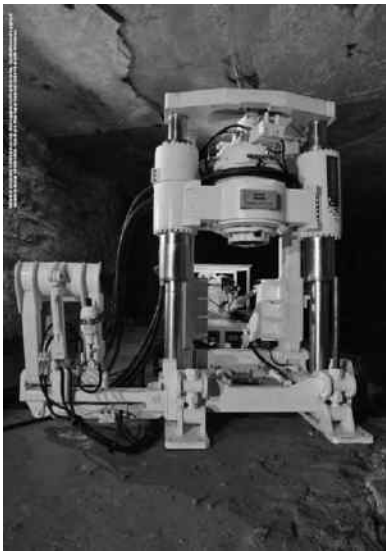
FIGURE 12.1 A raise boring machine. (Courtesy of Atlas Copco.)
