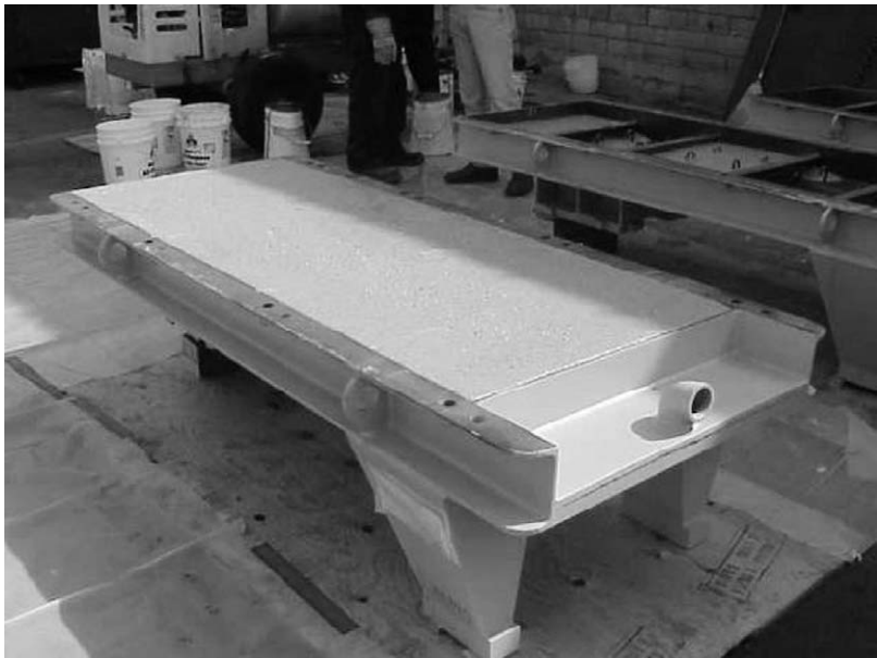
Figure 14-14. Pre-grouted pump base (bottom view).
