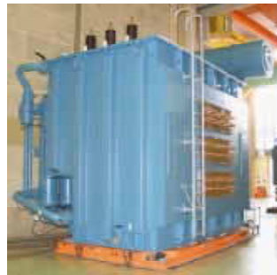
160 MVA steel EAF Transformer. Internal closure.
