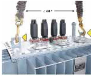
Transformer lifting example
