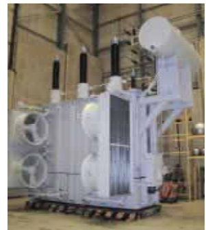
64 MVA Drives Converter Transformer. 12 pulse
