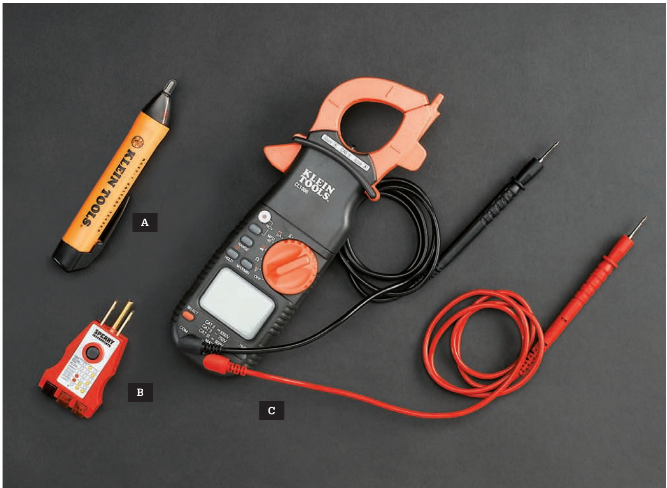
Diagnostic tools for home wiring use include: Touchless circuit tester (A) to safely check wires for current and confirm that circuits are dead; Plug-in tester (B) to check receptacles for correct polarity, grounding and circuit protection; Multimeter (C) to measure AC/DC voltage, AC/DC current, resistance, capacitance, frequency and duty cycle (model shown is an auto-ranging digital multimeter with clamp-on jaws that measure through sheathing and wire insulation).
