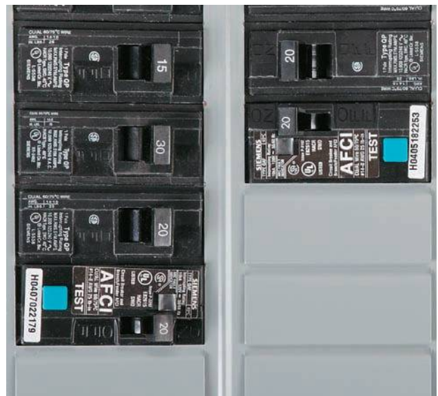
A combination ARC-fault circuit breaker detects sparking (arcing) faults along damaged energized wires and detects these faults between wires. A branch ARC-fault circuit breaker only detects arcing faults between wires.
