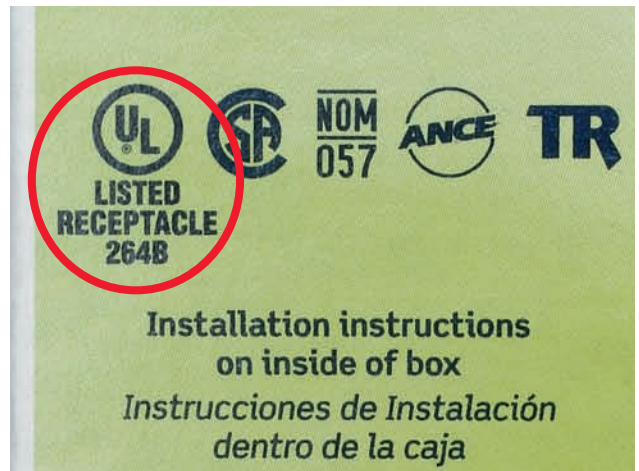
Use only UL-approved electrical parts or devices. These devices have been tested for safety by Underwriters Laboratories.
