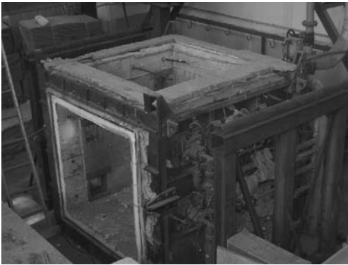
Figure 5. Standing / horizontal fireproof test furnace (1.15 m × 1.15 m).
