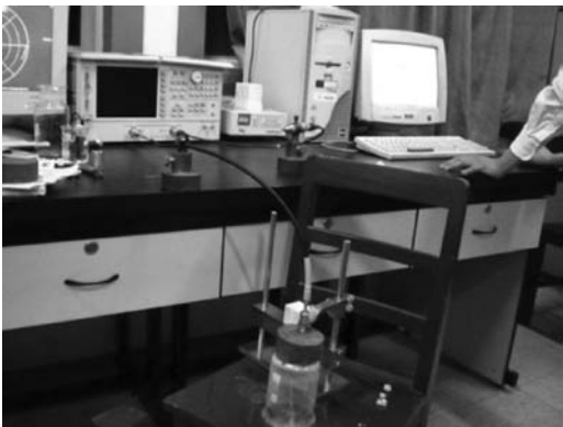
Figure 9. The dielectric constant testing of soil.
