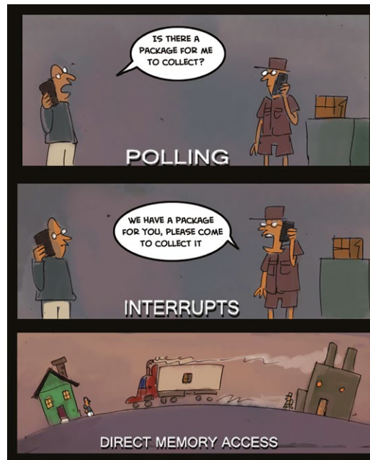
Figure 8.4: Parcel delivery analogy for IO transfer mechanisms. Image owned by the author.
