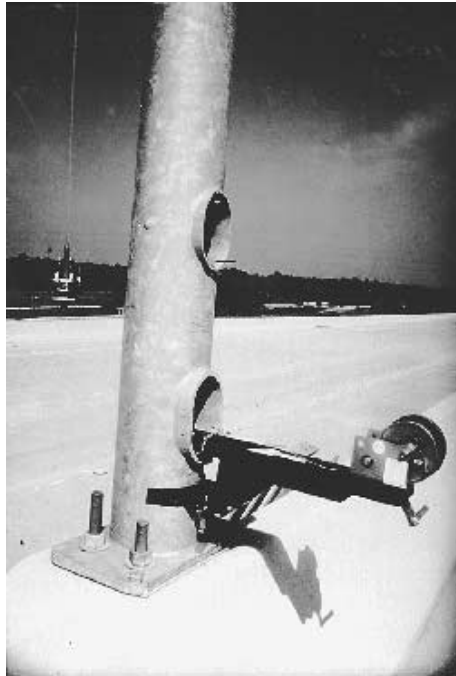
FIGURE 7.76 Lowering device manufactured by ITS Products Inc.
