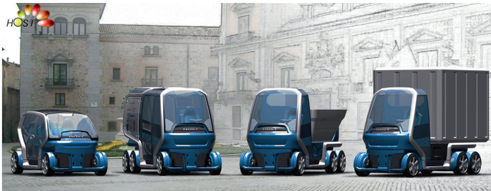
Figure 22.53 HOST: four services for one chassis (see color plate 9).
