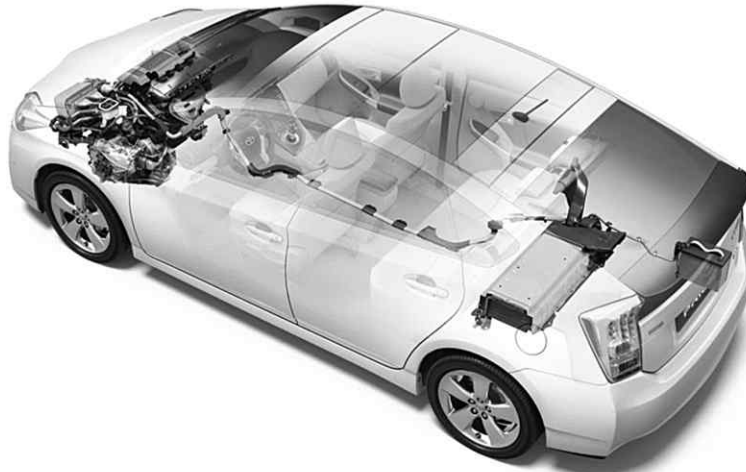
Figure 22.6 Third-generation 2010 Toyota Prius: hybrid system layout.
