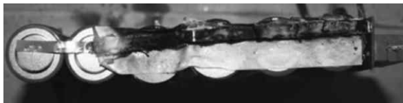
Figure 18.6 A short circuit failure in a multicell Li-ion battery.
