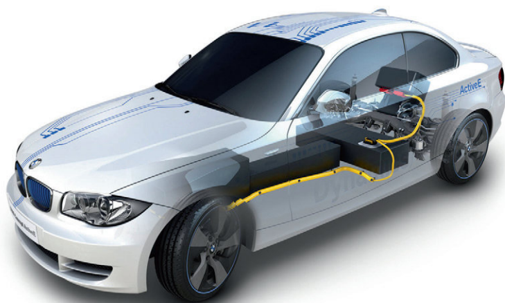
Figure 22.38 BMW Concept ActiveE: system layout (see color plate 8).
