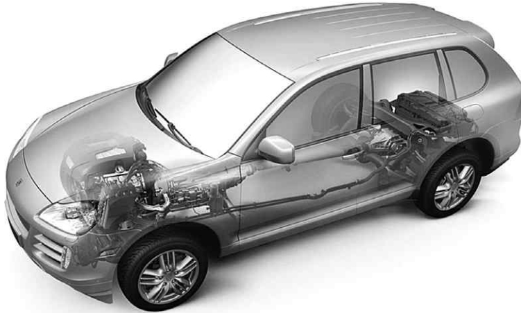
Figure 22.15 Porsche Cayenne Hybrid: system layout.
