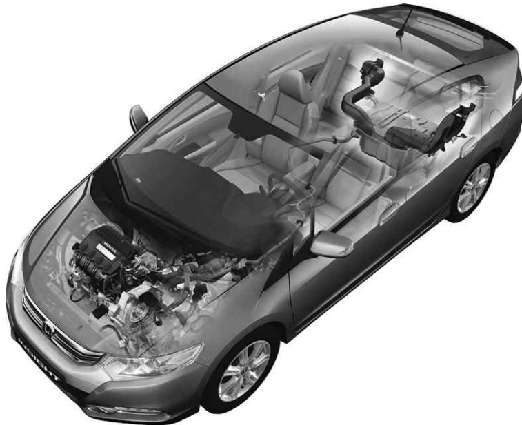
Figure 22.2 2010 Honda Insight: hybrid system layout.
