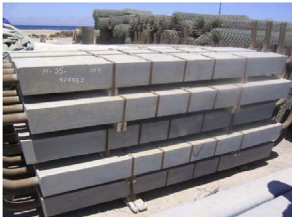
FIGURE 6.9 Cow horn anode weighing 189 kg.
