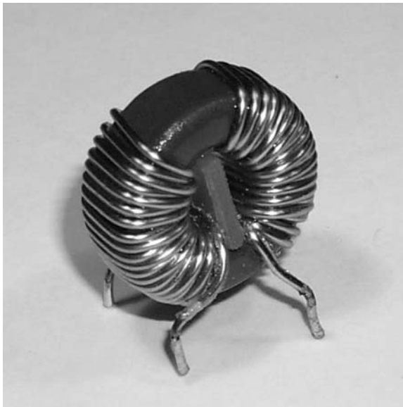
Figure 24.6: A 1:1 ratio toroidal transformer that forms part of a noise filter connected in the input circuit of a switched mode power supply
