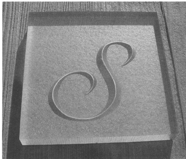
FIGURE A-11 Lettering reverse-engraved into 1/2-in acrylic.
