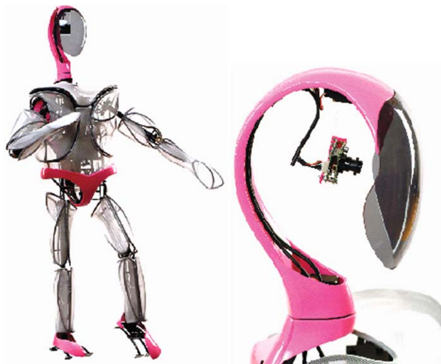
Figure 2.15. A full view and the head of the humanoid Lara. This robot is actuated by shape memory wire bundles, allowing significant weight reduction compared to robots with electric motors. Photo courtesy of Robert Kratz, Technical University of Darmstadt/HFG of Main, Germany.
