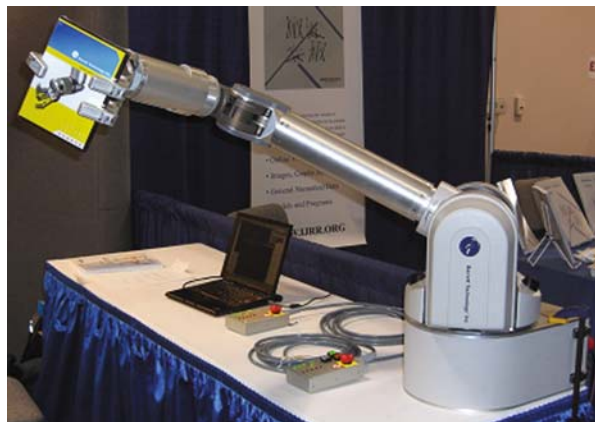
Figure 1.9. A robotic arm (made by Barrett Technology Inc.) is shown holding an object illustrating the biologically inspired operation of such manipulators. Photo by Yoseph Bar-Cohen at the 2008 IEEE International Conference on Robotics and Automation (ICRA) held in Pasadena, California.
