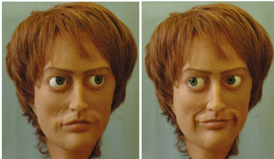
Figure 3.2. Using Frubber skin, a humanlike head that makes facial expressions was produced as a platform for testing artificial muscles.
