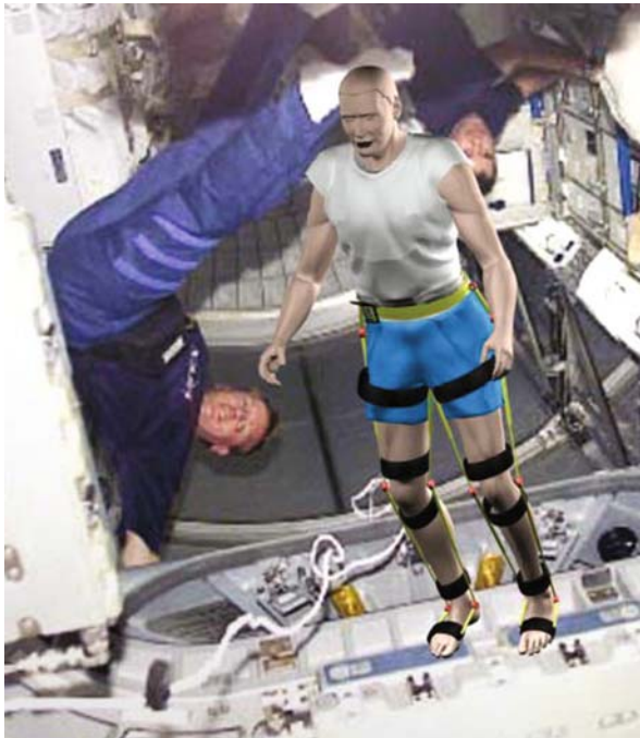
Figure 4.1. A graphic illustration of an exoskeleton concept for zero-gravity countermeasures, using an on-demand motion impeding system as a wearable exercise machine. The image of the robot with the exoskeleton is a courtesy of Constantinos Mavroidis, Northeastern University, Boston, Massachusetts. The background image of the two astronauts is a courtesy of NASA.
