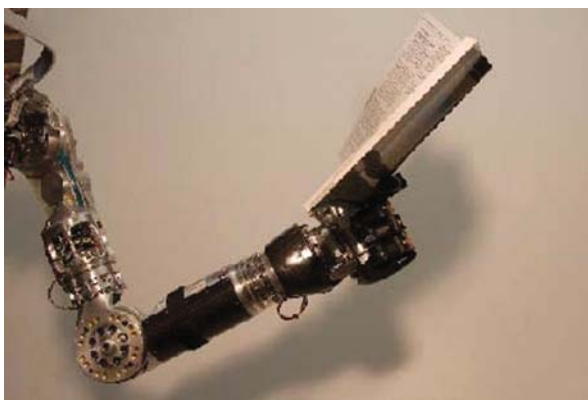
Figure 4.10. A humanlike arm holding a book in a reading pose, illustrating the ability to operate as an effective prosthesis. This arm was developed under the DARPA program Revolutionizing Prosthetics. Photo courtesy of Dirk Van Der Merwe, Deka Research & Development Corp., New Hampshire.
