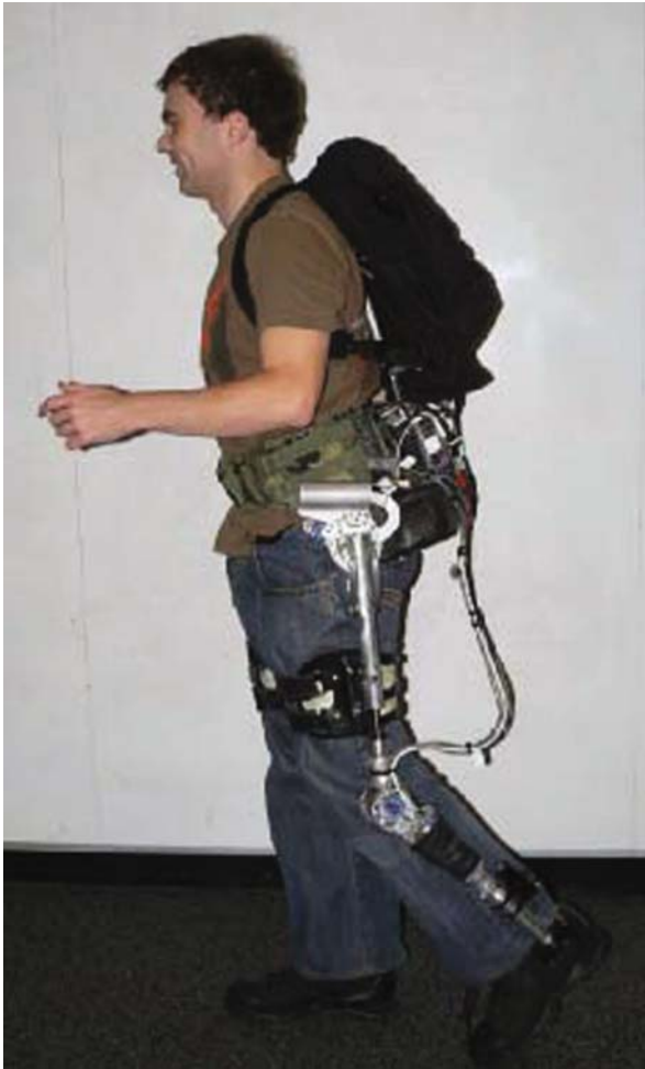
Figure 4.16. A motorless exoskeleton using variable damping in a passive system. Photo courtesy of Hugh Herr, Media Lab, MIT.
