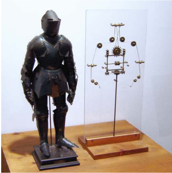
Figure 1.7. Model of Leonardo's robot and its inner working components. Photo is a public domain graphics courtesy of Wikipedia http://en.wikipedia.org/wiki/Image:Leonardo-Robot3.jpg
