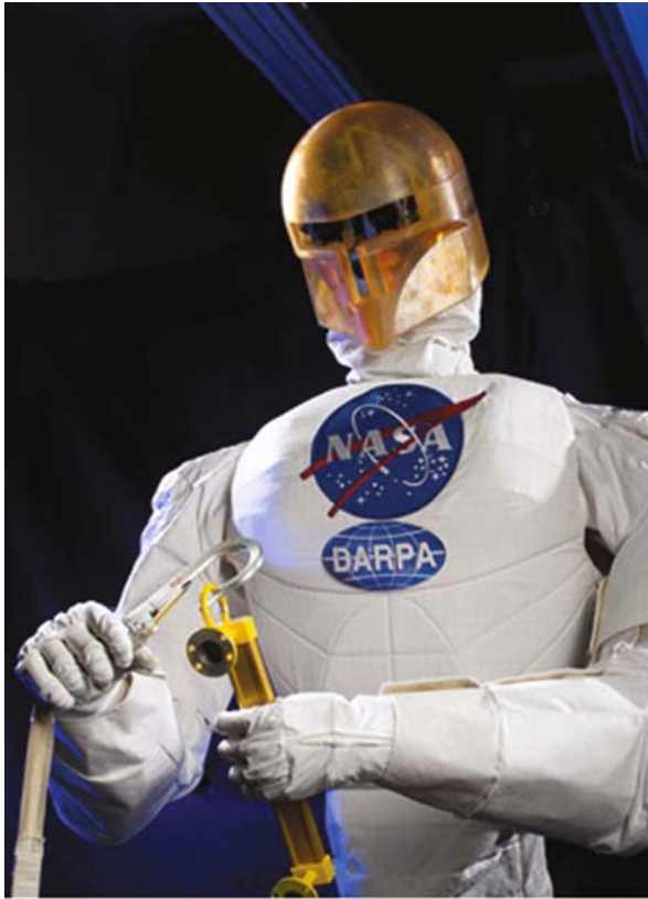
Figure 1.11. The humanlike robot called Robonaut is capable of performing manipulation tasks via human tele-presence control. Photo courtesy of NASA Johnson Space Center, Houston, TX.
