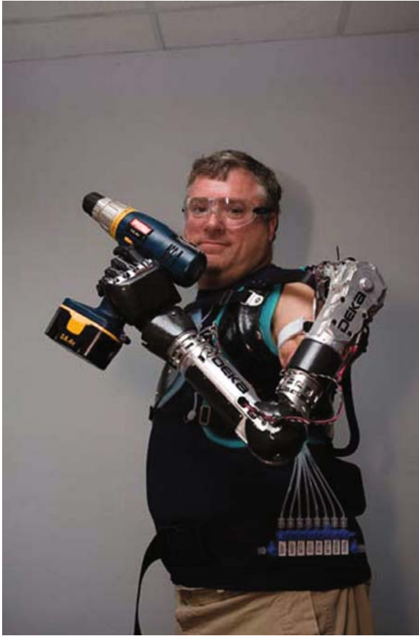
Figure 4.11. A prosthetic arm that is controlled by mirroring movements of the wearer's severed arm and the torso. This arm was developed under the DARPA. Photo courtesy of Dirk Van Der Merwe, Deka Research & Development Corp. New Hampshire.
