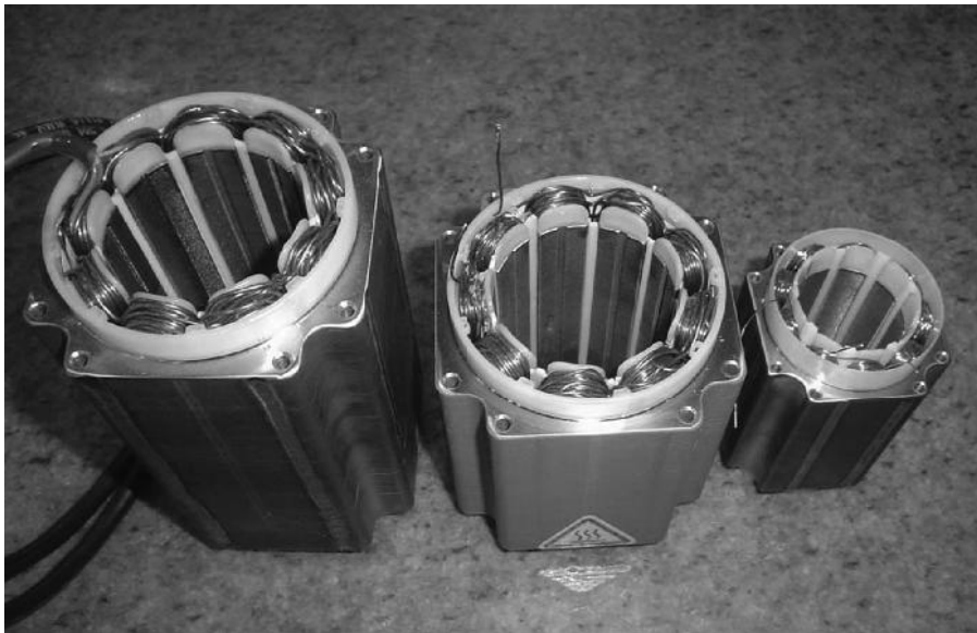
FIGURE 4.22 A variety of molded plastic insulators applied to stator windings.
