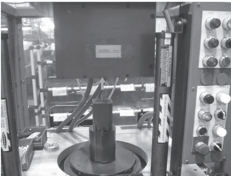
FIGURE 2.11 Postmagnetizing of a PM motor by means of a magnetizer.
