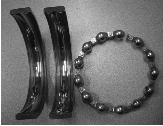
FIGURE 6.39 Bearing is cut for inspecting bearing damage and wear condition.
