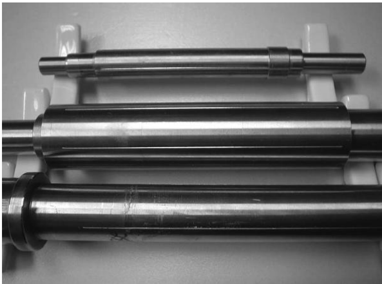
FIGURE 2.39 Serrations on motor shafts.
