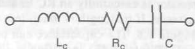
Figure 1.9 A chip capacitor is modeled as a series RLC circuit. Occasionally a shunt resistor is used to model dielectric losses, but this presents obvious problems at low frequencies.
